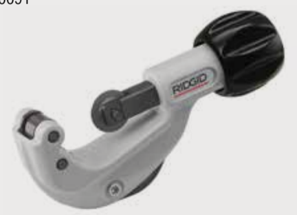
RIDGID 150 TUBE CUTTER 3-28MM 680091
