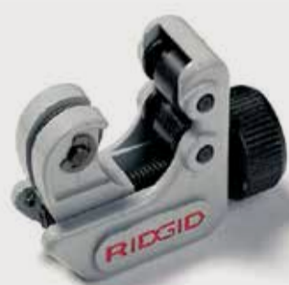
RIDGID 104 TUBE CUTTER 5-24MM 680084
